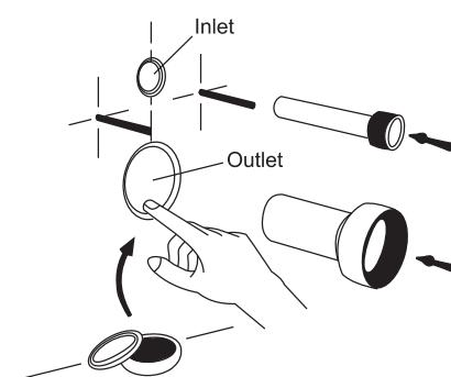
4. Connect the flush pipe and pan connector to the frame ready for connection to the toilet pan as shown, then screw the female threaded connectors (fixing bolts) onto the threaded bars so that the cut out aligns with the fixing hole in the toilet pan.
